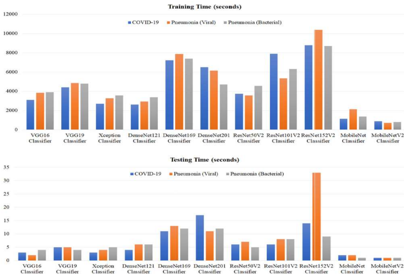
Fig. 3 Computation times including training and testing times for all deep learning image classifiers in this study
