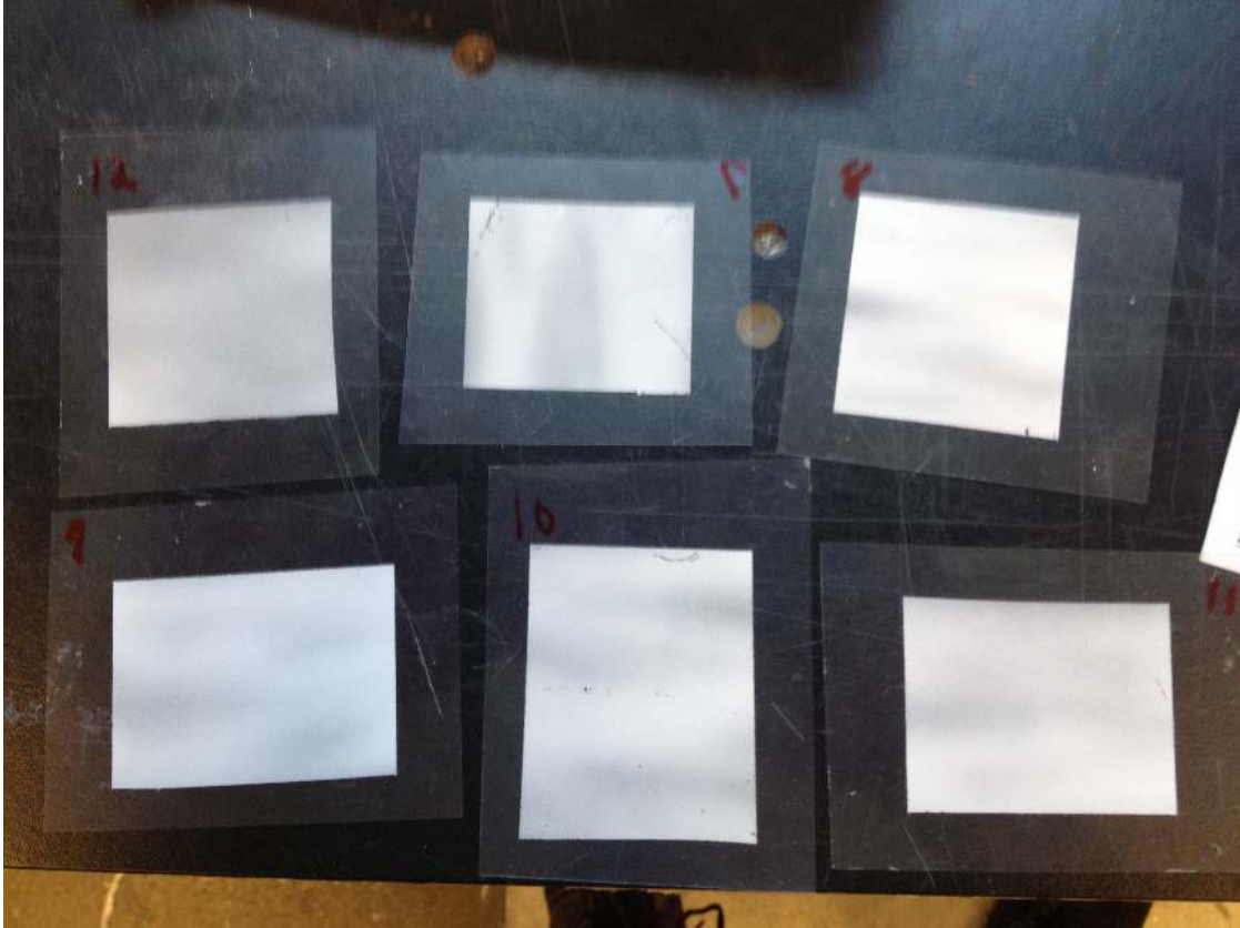
Figure 5.14: Painted BN squares on transparency sheets. Sheets were weighed before and after spraying to determine the approximate flow-rate of BN from the air gun.
