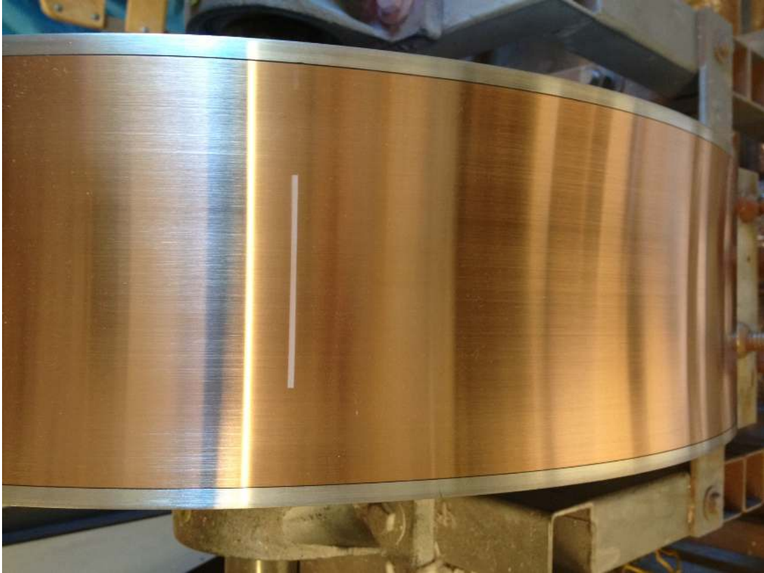
Figure 5.13: 1 mm wide BN stripe painted on the Cu-Be casting wheel as viewed from above the wheel.
