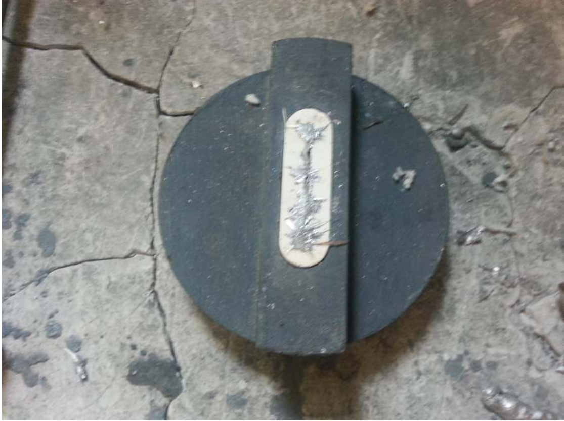
Figure 1.6: Nozzle cap seals the bottom of the crucible. During a cast, liquid metal flows through a ceramic insert (white piece) which fits in the nozzle. Insert shown here after a cast with frozen metal shards.
