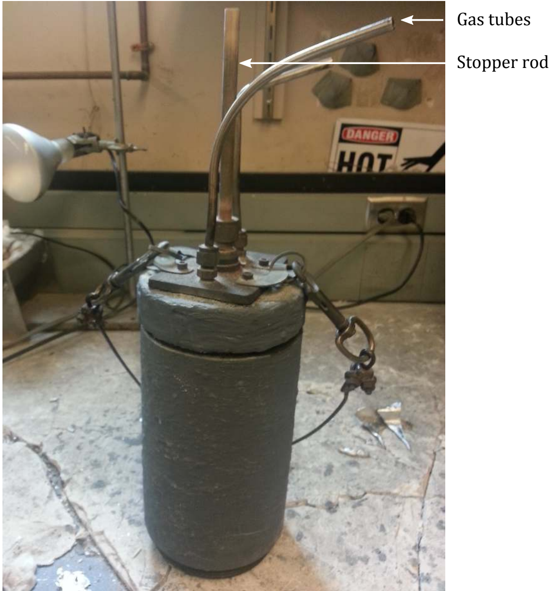
Figure 1.5: Assembled graphite crucible, with gas tubes and ceramic stopper rod.
