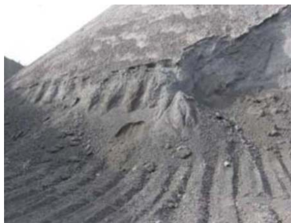
FIG. 7—Storage and maturation by hydration to air (Roque et al. 2007).
