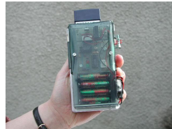
Fig. 7. PDA view from back showing location receiver hardware.
