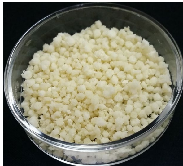
FIGURE 5 Urea coated with cassava starch-g-poly(acrylonitrile)
