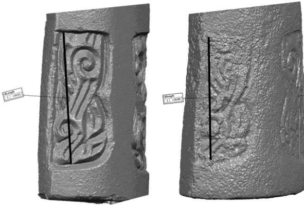
Figure 7. Illustration of how ornamental fields are measured on computerized 3D models to establish shrinkage. Detail of master model for fish-head pendant (left) and unfinished pendant (right), cf. Fig. 3D. Both scans conducted by the author
