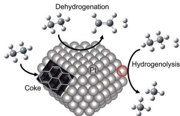
Fig. 3 Schematic image of reactivity of ethane on Pt particle. EDH proceeds on the Pt terrace sites, whereas coke formation and hydrogenolysis of ethane proceed on the "cus-Pt" sites circled in red.
