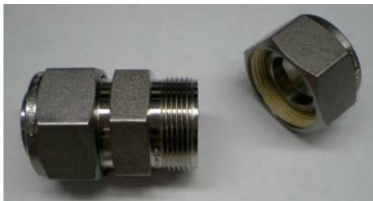
Figure 4. Photograph of 10 mL minireactors built from Swagelok junctions.
