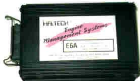
Figure 6. Haltech fuel injection controller.
