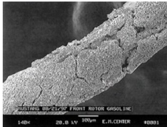
Figure 12. Igniter after catalyst breakdown.
