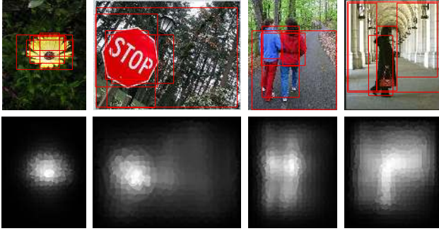
Figure 2. The top row shows sample images with the most confident 5 bounding boxes, with the bottom row the corresponding saliency map priors obtained from objectness.
