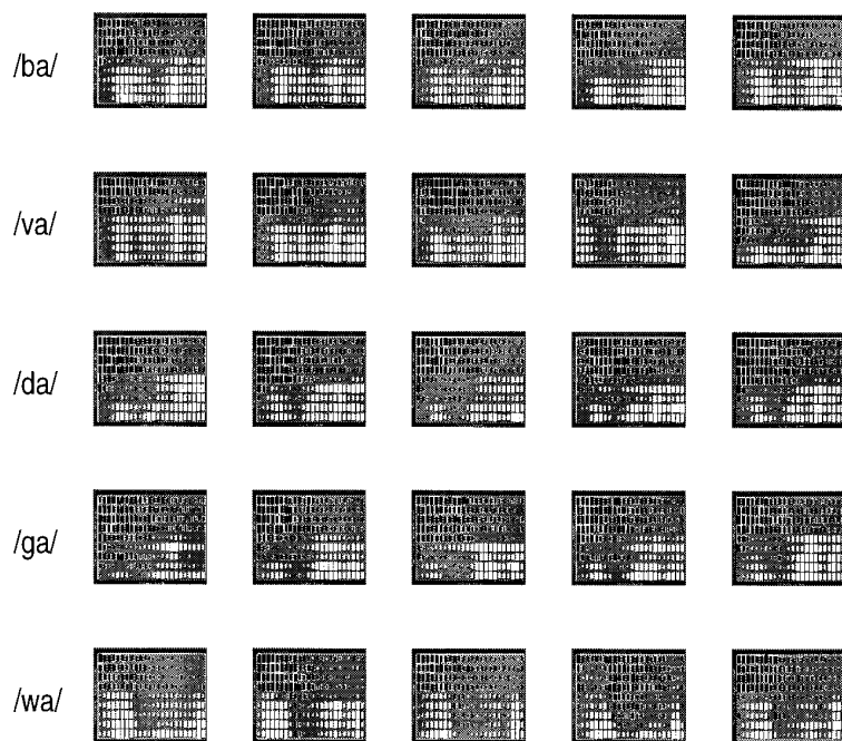
Figure 4: Example auditory patterns. The x -axis within each feature vector represents frequency channels and the y -axis time. The area of the small squares within the feature vector corresponds to the magnitude and the color that of the sign (white positive, black negative) of the feature dimension.
