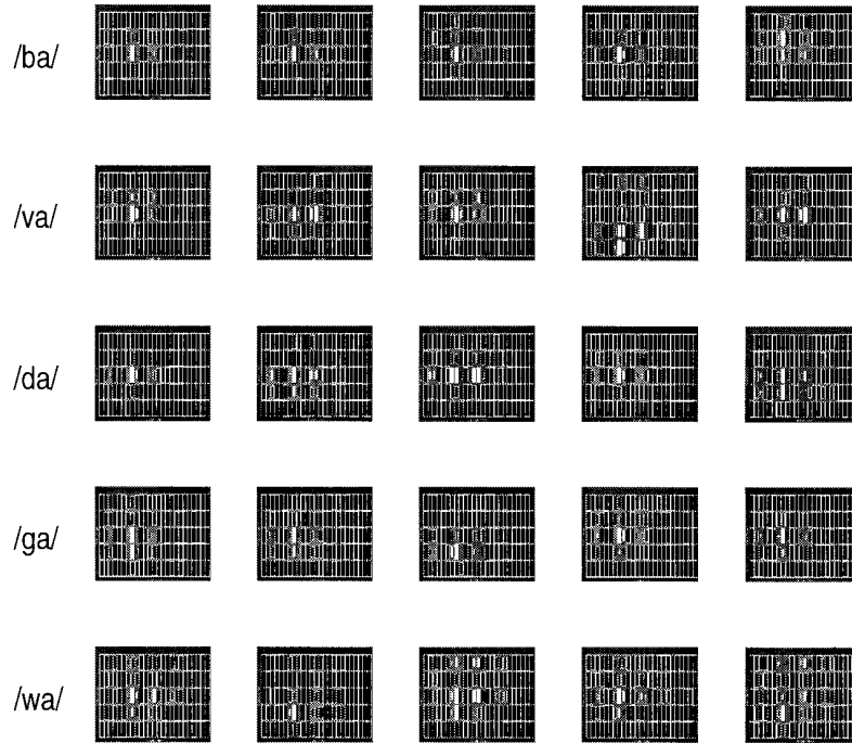
Figure 5: Example visual patterns. These patterns correspond to the auditory patterns in Figure 4. The x -axis represents spatial positions and the y -axis time. The area of the small squares within the feature vector corresponds to the magnitude and the color of the sign (white positive, black negative) of the feature dimension.
