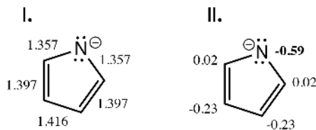
Figure 2: Bond lengths ( I. ) and Natural charges ( II. ) for anionic ( A^- ) calculated in \omega B97X-V/aug-cc-pVTZ. Charges indicated on carbon atoms are a sum of the C–H moiety. The aromatic nature of the ring leads to a planar structure with lengthened C_\alpha=C_\beta and slightly shortened C_\beta-C_\beta and C_\alpha-N (compared to pyrrole).
