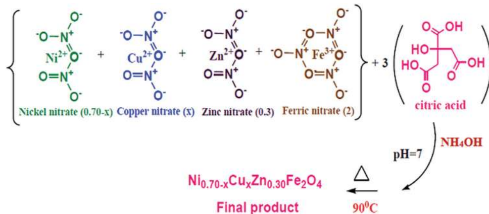
Fig. 2 Schematic of the mechanism of the \text{Ni}_{0.70-x}\text{Cu}_x\text{Zn}_{0.30}\text{Fe}_2\text{O}_4 ( x = 0.00, 0.05, 0.15, \text{ and } 0.25 ) synthesis.
