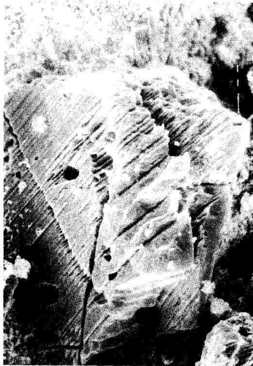
Figure 2. Calcite crystal from sample taken in the stucco shown in Figure 1. Etching, biological dissolution and pitting is evident. Bar represents 10 \mu\text{m} .
