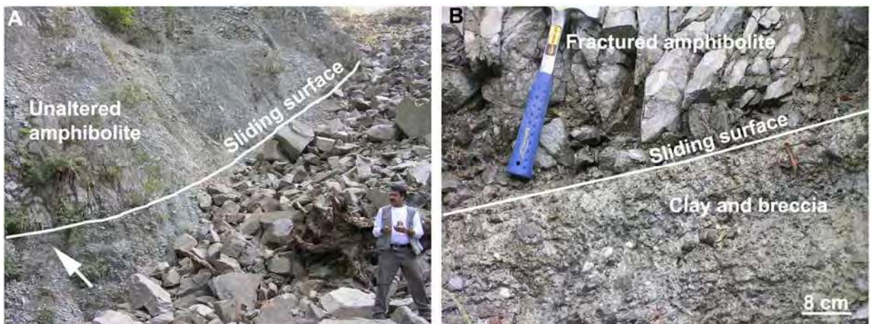
Fig 11, Large-scale landslide at Location 16 along Narayanghat-Mugling Road and close view of slip surface and altered clay zone. Arrow in Fig A shows the location of Fig B.
