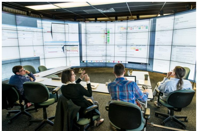
Figure 9. CAVE2 running in full 2D mode through SAGE. With a diameter of more than 10 feet, CAVE2 is big enough to fit about 15 standing users, and can be easily turned into a small meeting room.
