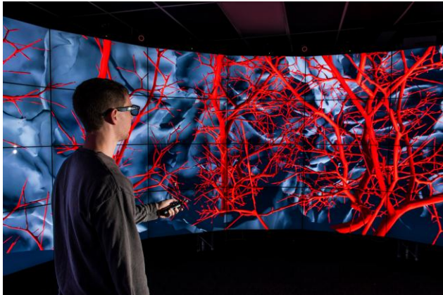
Figure 6. CAVE2 running in full 3D mode. The visualization shows reconstructed brain vessels and cortical tissue gathered from MRI data, supplemented with artificially generated microvasculature. Effective display of the finer details of this dataset is possible thanks to CAVE2 resolution.
