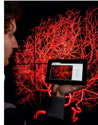
Figure 13. The Porthole interface running on a tablet device, displaying vasculature data rendered on the CAVE2 cluster.
