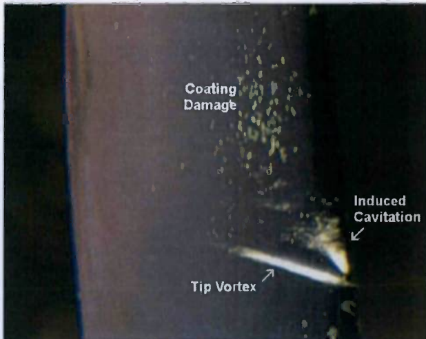
Figure 9 Overview of tip vortex cavity over the test foil with induced cavitation at the leading edge and resulting erosion damage (Mooney et al. [17]).
