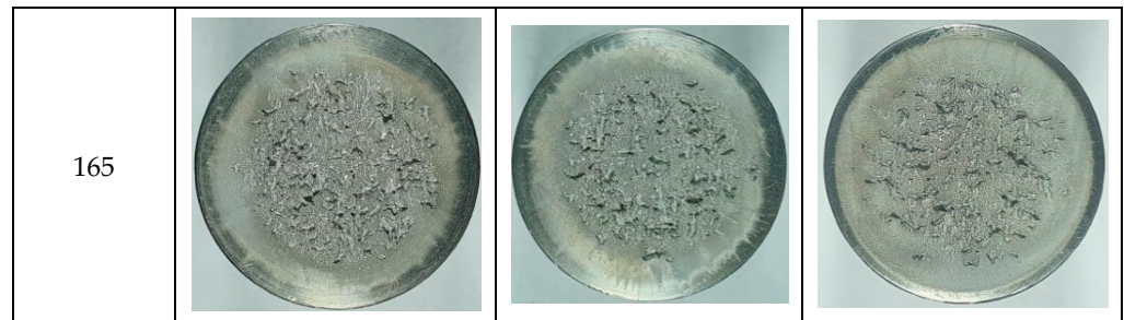
Figure 9. Macrographic images of the surface in cavitation tests of variable durations.
