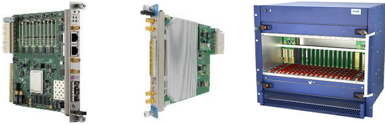
Figure 4.3 MicroTCA compliant for a typical LLRF system. Left: Digitizer SIS8300-KU from Struck. Middle: Signal conditioning board DWC8VM1 from Struck. Right: 12-slot MicroTCA4 crate from ELMA. Photo Credit: Struck Innovative System GmbH, Elma Electronic Inc.
