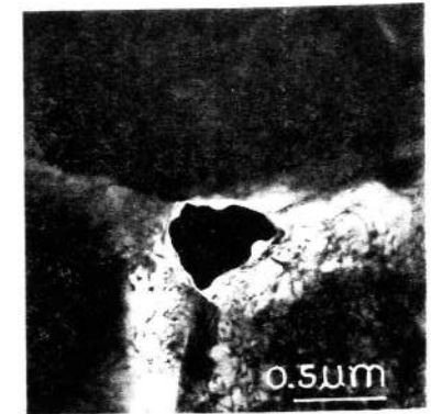
Fig. 8. Transmission electron micrograph of 7475 Al alloy fractured after a strain of 2.24.
