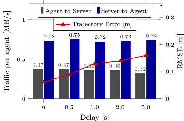
Figure 7: The influence of network delays enforced by the communication controller on the network traffic per agent and the trajectory error of the server map , using MH01.
