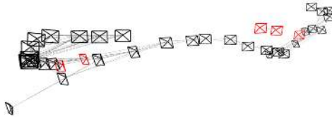
(c) Local map from Agent 1, with newly received KFs from the server to augment the local map colored in red.
