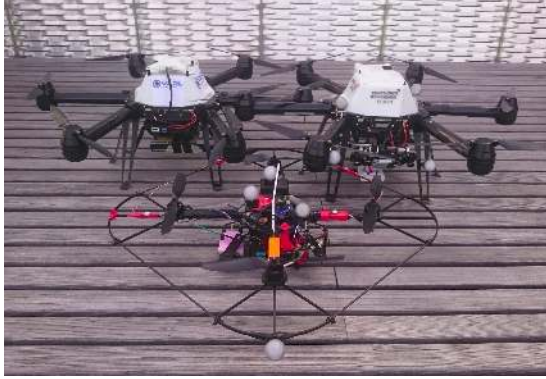
Figure 1: The UAV platforms used for our experiments: Two AscTec Neos with payload of 2 kg and one AscTec Hummingbird (middle) with payload of 200 g.
