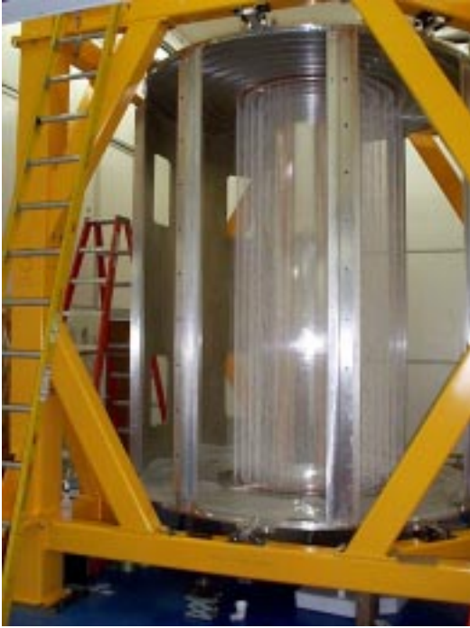
Figure 9. Alignment Fixture with the end plates, inner cylinder, and partial outer cylinder (reinforced staves, and two cover plates). Some pre-string lines are installed.
