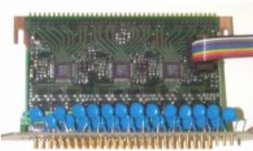
Figure 23. The ASDQ daughter board is shown inserted into the ASDQ motherboard. The three ASDQ chips are the largest ones on the daughter board.
