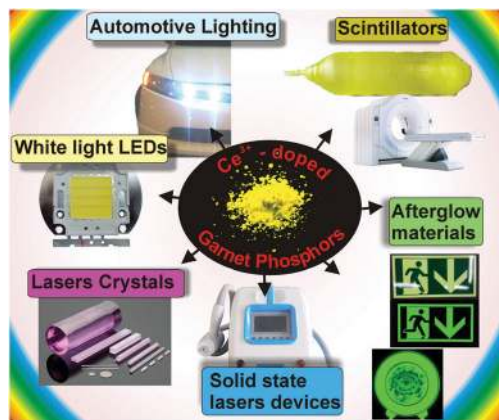
Fig. 2 Some representative application fields of \text{Ce}^{3+} -doped garnet phosphors including white light LEDs, scintillators, afterglow materials, laser crystals, and their corresponding applications.
