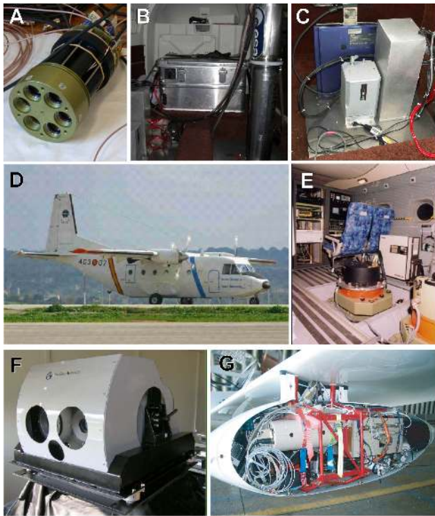
Fig. 3. Airborne instruments that were employed during the campaign to quantify changes of photosynthetic efficiency from the field to the regional level. (A) Internal sensor head of the AirFLEX sensor showing the six channels for O 2 -A and O 2 -B fluorescence retrieval. Each channel requires three spectral bands: within the atmospheric absorption feature and on the left and right shoulder of the absorption feature. (B) Picture of AirFLEX installed on board the CNR SENECA during the campaigns. (C) Thermal camera on board the SENECA. (D) INTA C-212-200 EC-DUQ “Paternina” aircraft. Within this aircraft both the AHS and HYPER sensor were installed for parallel recording of flight lines. (E) AHS hyperspectral imager onboard EC-DUQ “CASA” as arranged during the CEFLES 2 campaign. (F) Picture of the SIM.GA HYPERS sensor, which was first time used during the CEFLES2 campaign. (G) Underwing pod with the FieldSpec hyperspectral reflectance instrument. The instrument continuously acquired spectra with 2 Hz resolution along repeated overpasses during the campaign. The same, cross-calibrated detector was used on the ground (Fig. 2h).
