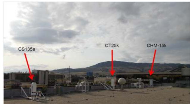
Figure 1. Ceilometer locations on CNR-IMAA Potenza observatory roof.
