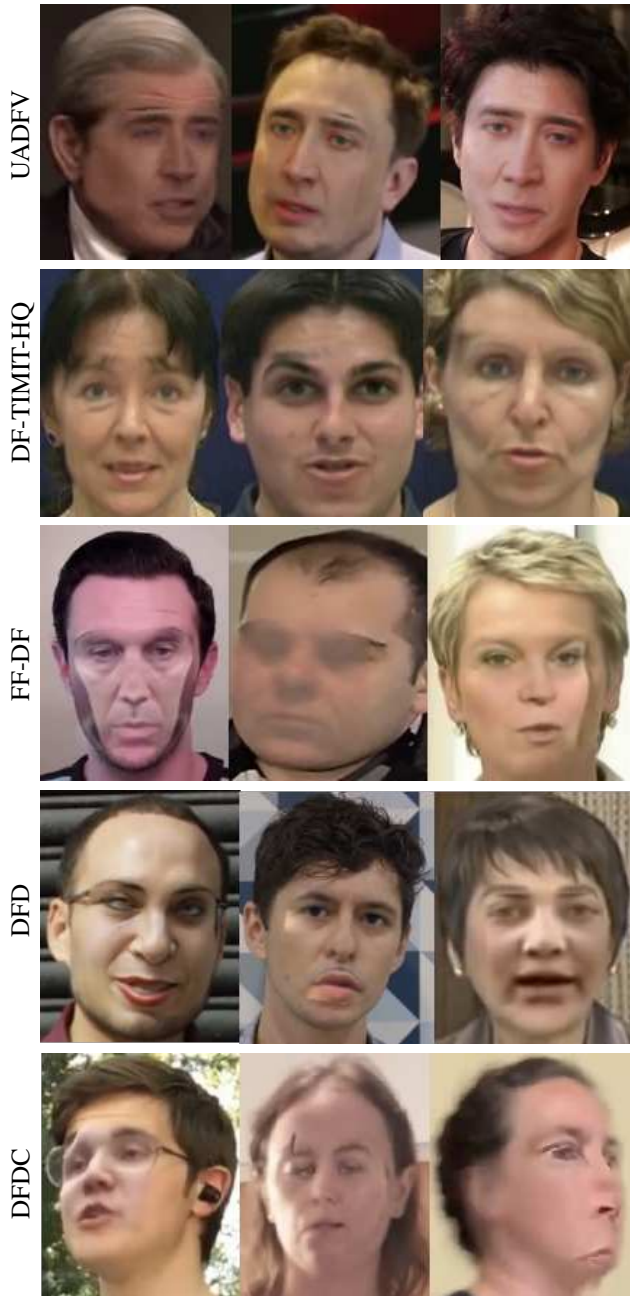
Figure 1. Visual artifacts of DeepFake videos in existing datasets. Note some common types of visual artifacts in these video frames, including low-quality synthesized faces (row 1 col 1, row 3 col 2, row 5 col 3), visible splicing boundaries (row 3 col 1, row 4 col 2, row 5 col 2), color mismatch (row 5 col 1), visible parts of the original face (row 1 col 1, row 2 col 1, row 4 col 3), and inconsistent synthesized face orientations (row 3 col 3). This figure is best viewed in color.
