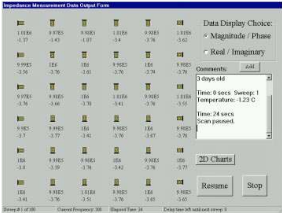
Figure 5.17: Display screen during measurements showing a schematic of the electrode array and the corresponding impedance. Comments could be added at any time.
