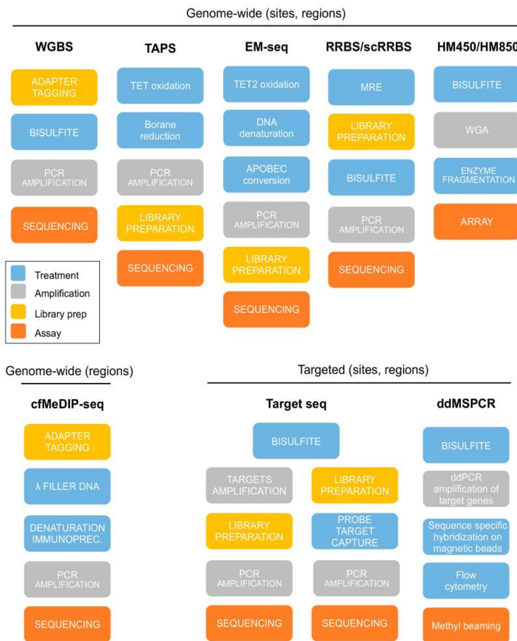
Figure 2. Summary of the experimental assays for DNA-methylation evaluation. Genome-wide techniques include methods able to perform site and region wise analysis, such as whole genome bisulfite sequencing (WGBS), TET-assisted pyridine borane sequencing (TAPS), enzymatic methyl-sequencing (EM-seq), reduced representation of bisulfite sequencing (RRBS, single-cell RRBS (scRRBS)), and infinium methylation arrays (HM450, HM850), and methods analyzing DNAm regions only, such as circulating free methylated DNA immunoprecipitation sequencing (cfMeDIP-seq). Targeted methods include target bisulfite sequencing (target bisulfite seq) and PCR-based assays, including methylation specific PCR (MSPCR) and droplet digital methylation specific PCR (ddMSPCR). MRE: methylation restriction enzyme, WGA: whole genome amplification.
