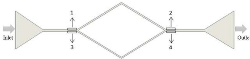
Figure 1 Schematic representation of the microchannel geometry and location of the sections where the images were collected and the CFL was measured
