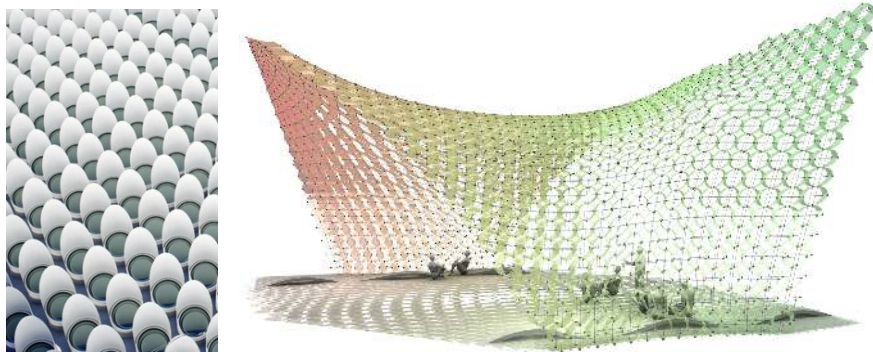
Figure 17: Indirect lighting by oblique cylinders (at left, High Museum of Art, Atlanta) motivates a shading system consisting of developables, created by a subdivision process.
