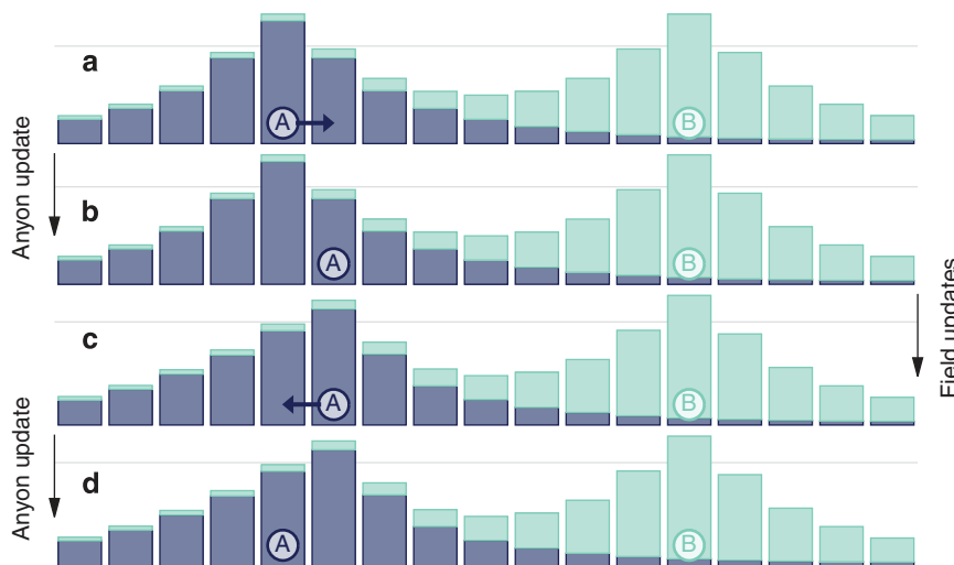
Figure 3. Self-interaction. A setup with two isolated anyons A and B , and their fields in a self-interaction cycle. Suppose that the fields from each anyon starts in its stationary configuration (a). After one anyon update move, anyon A moves in the direction of largest field gradient towards anyon B . (b) Immediately after anyon A moves, the field which it leaves behind is much larger than the field from anyon B . (c) After a certain number of field updates, the residual self field from anyon A decreases, but might still tell the anyon to move in the wrong direction (d).
