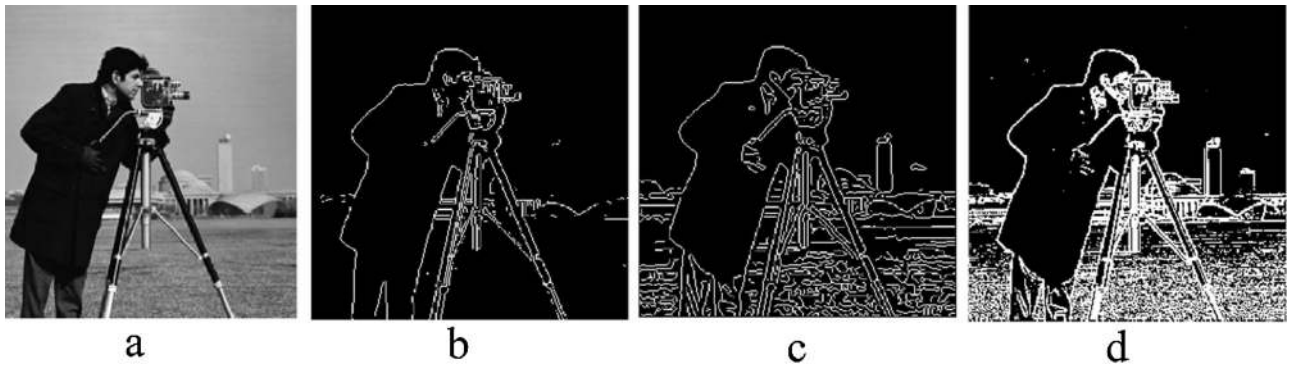
Fig. 8. (a) The Cameraman test image, (b) Prewitt algorithm, (c) Canny algorithm and (d) CED algorithm.
