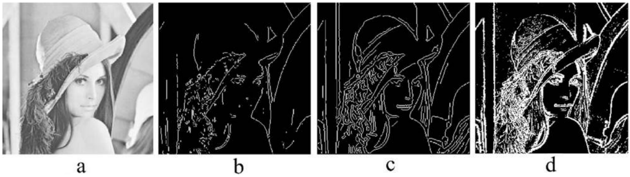
Fig. 7. (a) The Lena test image, (b) Prewitt algorithm, (c) Canny algorithm and (d) CED algorithm.
