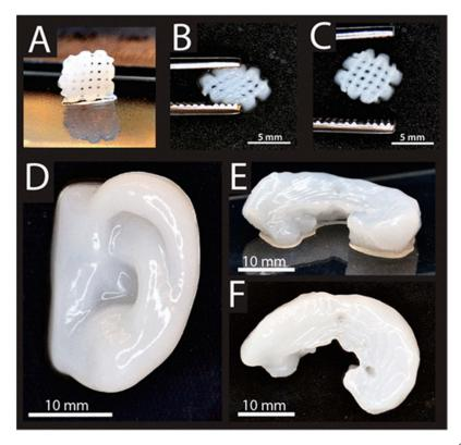
Figure 12. The 3D printing of NFC-alginate into (A) small grids  $(7.2 \times 7.2 \text{ mm}^2)$ , (B) after squeezing, and (C) restored after squeezing; (D–F) 3D-printed human ear in different views. Reprinted with permission from Ref. [280]. 2015, ACS.
