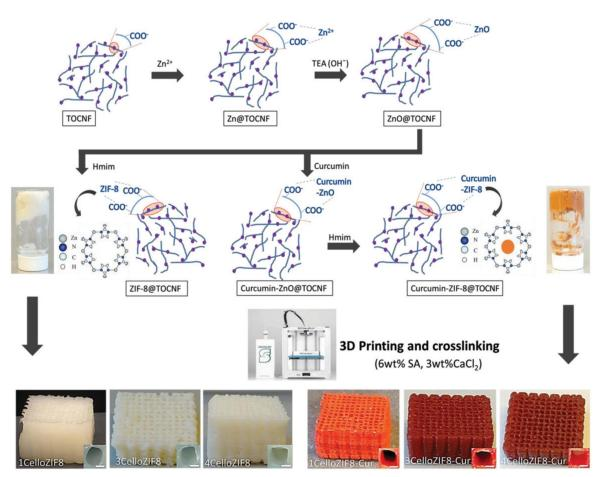
**Figure 10.** The synthesis procedure of cellulose-ZIF8 bioink and their processing into the 3D network via 3D printing. Reprinted with permission from Ref. [248]. 2019, John Wiley & Sons.
