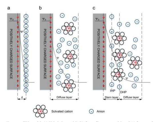
**Figure 3.** EDL model, (**a**) Helmholtz model, (**b**) Gouy–Chapman model, and (**c**) Stern model. Reprinted with permission from ref. [1]. 2016 Elsevier.
