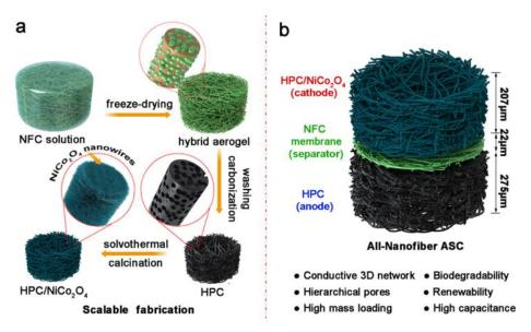
**Figure 6.** Schematic representation of the (**a**) fabrication of nanocellulose-derived HPC and HPC/NiCo<sub>2</sub>O<sub>4</sub> composite aerogels and (**b**) their asymmetric assembly into an all-nanofibre ASC device. Reprinted with permission from ref. [112]. 2019 American Chemical Society.
