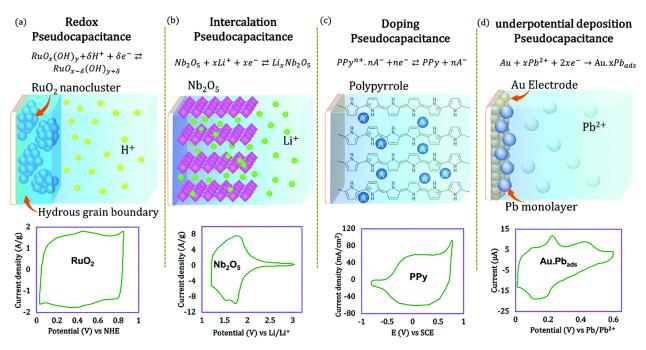
**Figure 4.** Different type of pseudocapacitances and the nature of the cyclic voltammetry (CV) curve. Reprinted with permission from ref. [22]. 2019 American Chemical Society.
