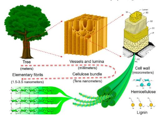
**Figure 5.** Schematic illustration of hierarchical structure of wood, from macroscopic to molecular level. Reprinted with permission from ref. [71]. 2018 American Chemical Society.
