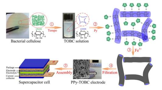
**Figure 8.** Schematic process of the fabrication and layered structure of supercapacitor cell. Reprinted with permission from ref. [124]. 2016 Elsevier.
