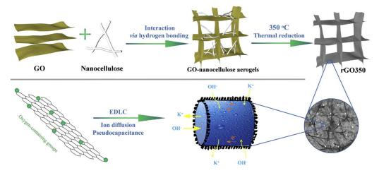
**Figure 7.** Schematic representation of the synthesis and ionic and electronic transport research mechanisms of rGO aerogel as a capacitor electrode within a KOH electrolyte. Reprinted with permission from ref. [115]. 2017 Elsevier.
