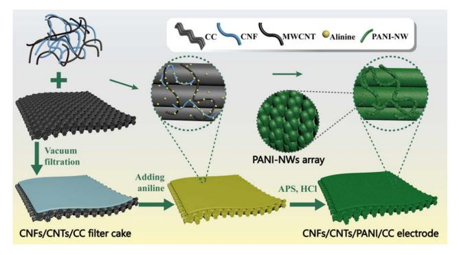
**Figure 9.** Schematic of the preparation process of CNFs/CNTs/PANI-NW/CC electrodes. Reprinted with permission from ref. [152]. 2018 IOP Publications.
