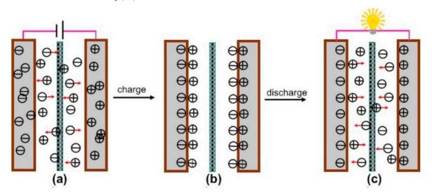
Figure 2. Schematic illustration of the charging process (a): charged state (b), discharging process (c) [26].
