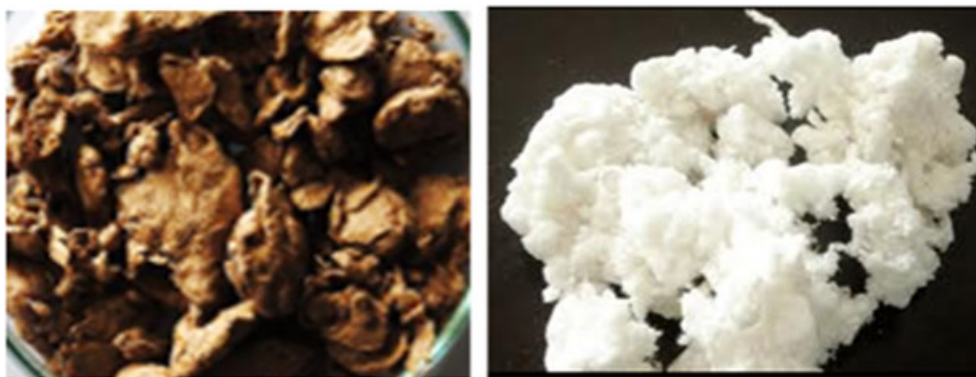
Figure 1. The raw materials used to obtain CNCs: Cotton linters (right), kraft pulp from hardwood (left).
