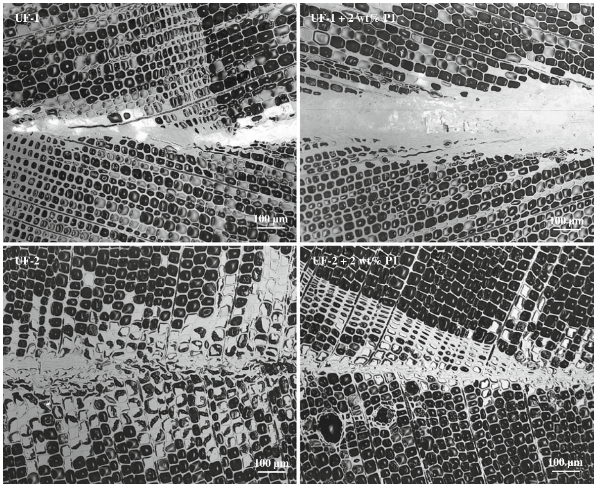
Fig. 4 Optical micrographs of urea-formaldehyde-(UF) bond lines. Two different adhesives were applied, once without any additional filler (UF-1 and UF-2) and once filled with 2 wt%
