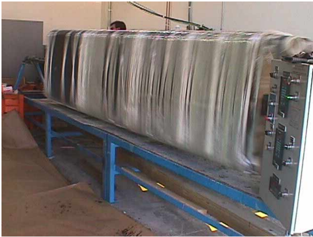
Figure A7. The solar car team designed a composite chassis of E-glass fiber wound on aluminum honeycomb. This picture shows the chassis being wound on the composite winding machine.
