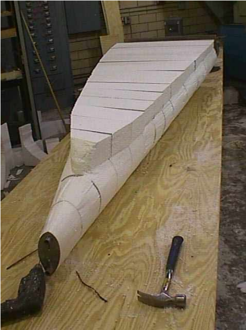
Figure A2. Concrete Canoe mold of Styrofoam taking shape.
