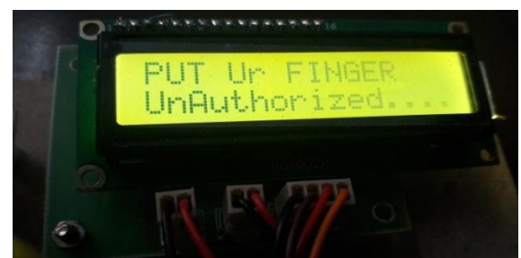
Person swipe card it shows authorized card and GSM sends sms to user mobile authorized card then person give fingerprint and database shows unauthorized fingerprint because his fingerprint is enrolled in database
