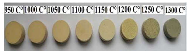
Fig. 4. Ceramic samples sintered at different temperatures
