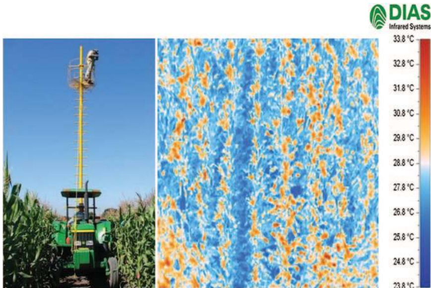
Fig. 13.10 Thermal images of tropical maize on rows taken at the CIMMYT station of Tlaltizapan (Mexico). Emitted long-wave infrared radiation is processed into color digital image display of the different temperatures in the target area
