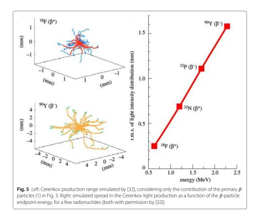
in color indicates the point where the energy of the particles goes below the Cerenkov threshold. The right part of the figure shows the root mean square spread of the Cerenkov light production for a few radioisotopes, plotted as a function of the endpoint energy of the  $\beta$ -particle.
