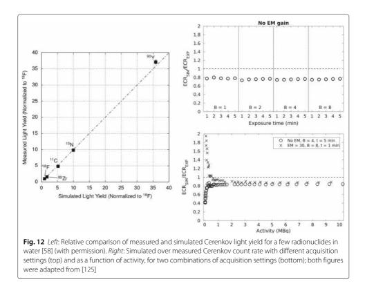
different acquisition settings (e.g., varying the pixel binning factor and exposure time, top) and different activity levels (bottom), provided that the activity was above the minimum radioisotope activity level that can be detected with CLI. Additional measurements with tissue samples and emission filters to separate Cerenkov spectral components are being carried out to confirm these preliminary results.
