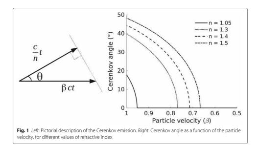
The Cerenkov threshold can be expressed in terms of the kinetic energy of the charged particle with the following equation (using  $E = T + m_0 c^2 = \gamma m_0 c^2$ ):
