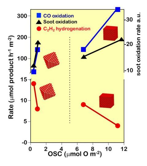
**Figure 12.** Rate of CO and C-soot oxidation and  $C_2H_2$  hydrogenation against OSC as measured in polyhedral and cubic shaped nanoparticles. Adapted from ref. 147. Copyright (2014), with permission from John Wiley and Sons.
