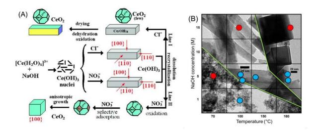
**Figure 6**. Left: schematic illustration for the conversion from nanorods to nanocubes; Adapted with permission from ref. 86. Copyright (2008) American Chemical Society. Right: morphological phase diagram of CeO<sub>2</sub> after hydrothermal treatment. Red circles refer to the original points while blue circles are values taken from the literature; Adapted with permission from ref. 88. Copyright (2013) Elsevier.
