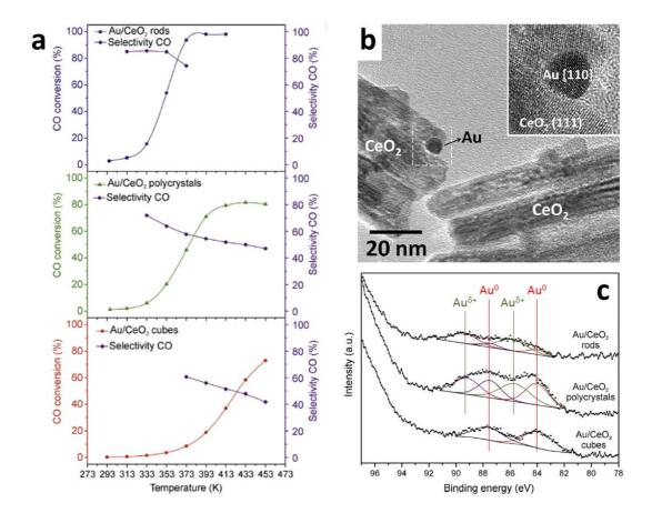
**Figure 18.** A. COPrOx catalytic performance of preformed Au nanoparticles dispersed over ceria nanopolyhedra, nanocubes and nanorods ( $CO:O_2:N_2:H_2=1:1:23:25$  molar); B. HRTEM image of Au/Ceo<sub>2</sub> nanorods; C. Au 4f photoemission spectra. Adapted with permission from ref. 181 Copyright 2016 Elsevier.
