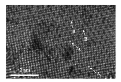
**Figure 19.** HAADF-STEM image recorded over  $Au/CeO_2$  containing Au single atoms (bright atoms indicated by A) and many clusters of Ce vacancies (indicated by B). The oxygen atoms are not visible under this imaging mode. Reproduced with permission from ref. 184. Copyright 2017 American Chemical Society.
