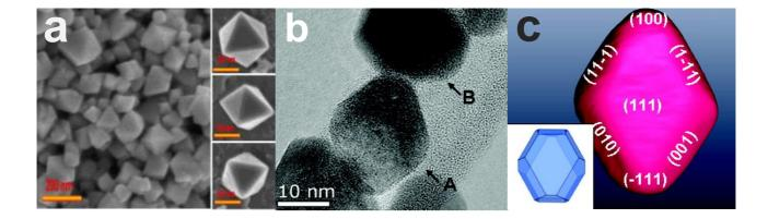
**Figure 4**. CeO<sub>2</sub> crystals prepared by hydrothermal methods: (a) FE-SEM image of CeO<sub>2</sub> nano-octahedrons and individual nano-octahedron seen from three different views. Adapted with permission from ref. 73. Copyright (2014) Elsevier. (b) Bright-field image of large CeO<sub>2</sub> particles and (c) surface 3D rendering view of the structure of particle A. Adapted with permission from ref. 72. Copyright (2011) American Chemical Society.
