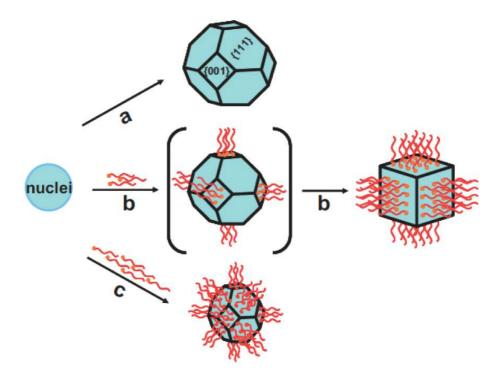
**Figure 5**. Control of nanocrystal shape through the use of surface capping agents. Interaction of dodecanoic acid with {100} surfaces slows the growth in this direction leading to formation of nanocubes (path b). In excess of dodecanoic acid, growth in both directions is reduced with formation of small truncated octahedral particles (path c) compared to path a with no capping agent. Adapted from ref. 77. Copyright (2007), with permission from John Wiley and Sons.
