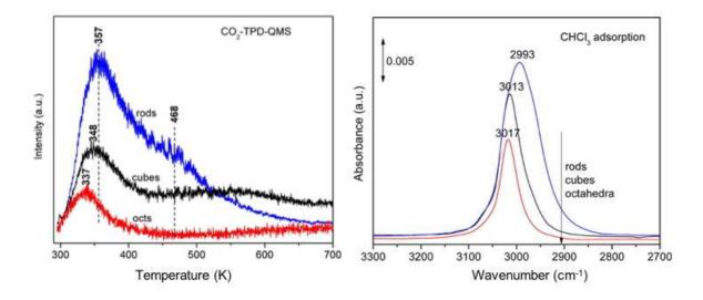
**Figure 13.** Left:  $CO_2$ -TPD profiles obtained over ceria nanoshapes (surface area normalized mass 44 signal); right: IR spectra from  $CHCl_3$  adsorbed at room temperature on ceria nanoshapes calcined at 673 K. Adapted with permission from ref. 152 Copyright 2015, American Chemical Society.
