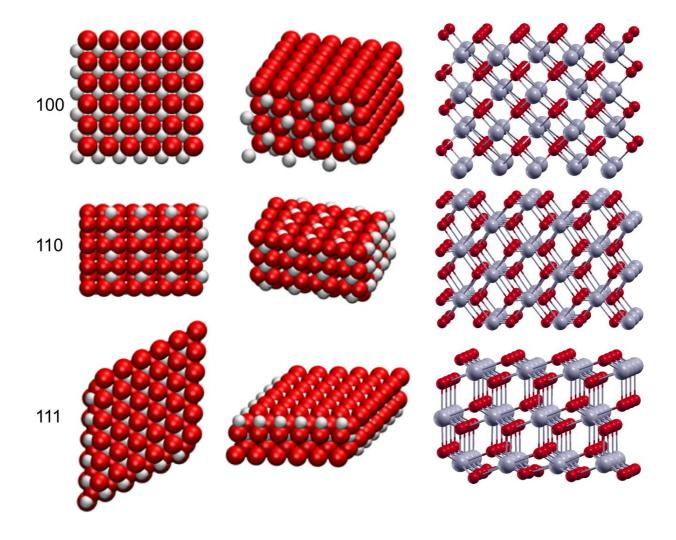
**Figure 1.** Top, side and perspective view of  $CeO_2$  (100), (110) and (111) surfaces. Gray and red spheres represent cerium and oxygen ions respectively.
