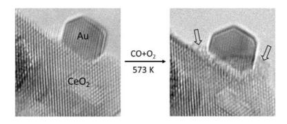
**Figure 16**. ETEM images recorded over Au/CeO<sub>2</sub>-nanorods. Under CO oxidation conditions a restructuration of the Au-CeO<sub>2</sub> interface occurred, resulting in disordered ceria layers adjacent to the Au nanoparticles. Adapted with permission from ref. 108. Copyright 2012 American Chemical Society.
