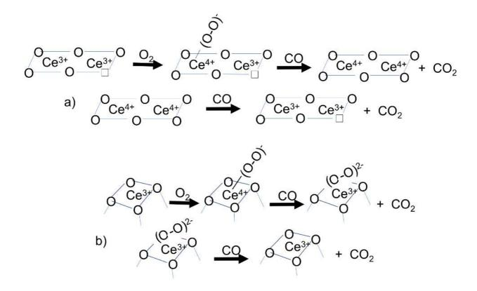
**Scheme 1.** (a) Reduction-oxidation cycle operated by  $CO/O_2$  over ceria surfaces in the presence of superoxide and  $Ce^{3+}$  with associated vacancy. CO reacts with superoxide formed by interaction at a top site of  $Ce^{3+}$  apart from an oxygen vacancy<sup>123</sup>. (b) Sketch of a conceivable reduction oxidation cycle operated by  $CO/O_2$  over small size ceria NPs in the presence of  $Ce^{3+}$  not associated with a vacancy and located in defect position.
