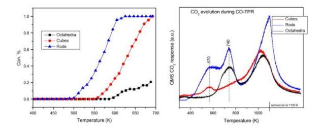
**Figure 11**. (left) Light-off curves for CO oxidation over ceria rods, cubes, and octahedra. Reaction conditions: catalyst  $\sim$ 50 mg, reaction feed: 10 mL/min 2%CO/Ar/He + 30 mL/min 5% O<sub>2</sub>/He. (right) CO<sub>2</sub> evolution during CO-TPR. Adapted from ref. 126. Copyright (2012), with permission from Elsevier
