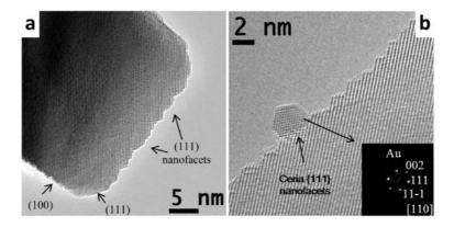
**Figure 17**. HRTEM images recorded over reconstructed  $CeO_2$  nanocubes with {111} nanofacets (a) and the corresponding Au/ $CeO_2$  catalyst (b). Au nanoparticles are preferentially located in the valley locations of the zigzagged {111} nanofacets of the ceria support. Adapted with permission from ref. 97. Copyright 2015 American Chemical Society.
