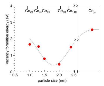
**Figure 3**. Size dependence of vacancy formation energy for different ceria nanoparticles. Data from ref. 63.
