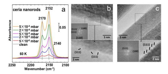
**Figure 10.** (a) CO adsorption on ceria nanorods with bands at 2170 and 2152 cm $^{-1}$  due to adsorption on {110} and {111} surfaces respectively (b,c). High-magnification HRTEM images of CeO $_2$  nanorods showing the {111} facets formed on the (110) plane. Adapted with permission from ref. 110. Copyright Wiley-VCH (2017).
