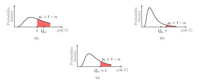
Figure 2: Illustration of equivalence of PoF (shown by the shaded region) and  $Q_{\alpha}$  showing that the two quantities converge at the constraint threshold when the reliability constraint is active.
