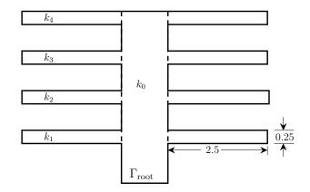
Figure 8: Fin geometry and model parameters.
