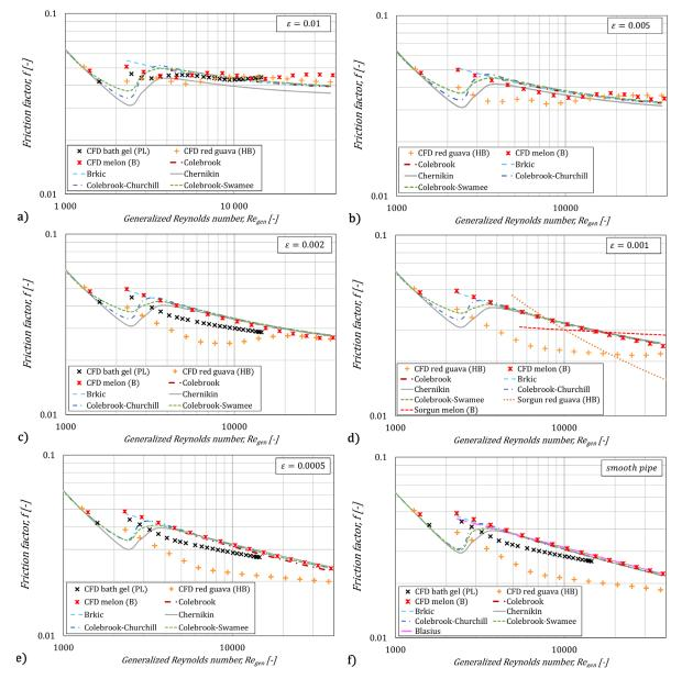
Fig. 6 Numerical and estimated friction factors with the bath gel (PL), the red guava pulp (HB) and the melon juice (B) in pipes with different roughness. a)  $\varepsilon = 0.01$ ; b)  $\varepsilon = 0.005$ ; c)  $\varepsilon = 0.002$ ; d)  $\varepsilon = 0.001$ ; e)  $\varepsilon = 0.0005$ ; f) smooth pipe
