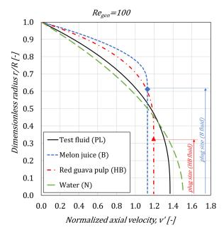
**Fig. 3** Normalized axial velocity profiles in smooth pipe for the powerlaw, Bingham, Herschel-Bulkley fluids and with water at Re<sub>gen</sub> = 100. Analytical dimensionless radius of the flow for the B( $r_{plug,B}/R = 0.612$ ) and HB( $r_{plug,HB}/R = 0.326$ ) fluids
