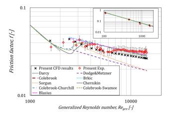
Fig. 5 Experimental (with error bar), numerical and predicted friction factors with the test fluid (PL) in smooth pipe
