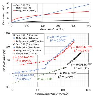
Fig. 4 Rheograms (top) and nominal shear rate-shear stress diagrams (bottom) in smooth pipe for the three investigated fluids in laminar and turbulent regimes; the analytical curve of Eq. (12) with the power-law fluid in laminar zone (green dotted)
