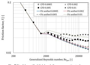
Fig. 7 Fit of the unified Colebrook-Swamee equation to the CFD results with the Bingham fluid for the rough pipes of  $\varepsilon = 0.01; 0.005; 0.002; 0.0005$
