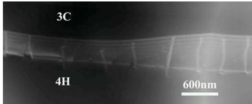
Fig. 9. TEM cross-sectional bright field image of the step-free 3C/4H interface with sample slightly tilted to reveal interfacial misfit dislocations. [27] Almost vertical line contrast corresponds to misfit dislocations at or near the 3C/4H interface plane. No dislocations were observed to propagate vertically into the 3C-SiC film.
