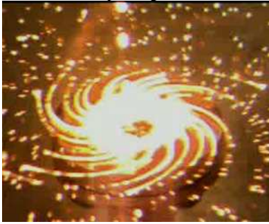
Figure 1: Typical still image from high speed video recording of the dry granulation at a spinning disc in CSIRO dry slag granulation process.
