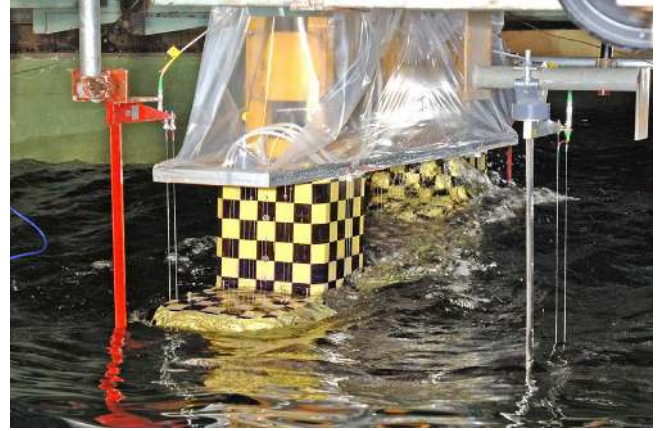
Figure 1. Experimental model, semi-submersible
