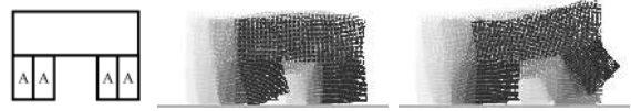
Fig. 4: A soft 2D walker with controller optimized using gradient descent, aiming to achieve a maximum distance after 600 simulation steps. The walker has four actuators (left, marked by letter ‘A’s) with each capable of stretching or compressing in the vertical direction. The full walking animation (middle and right) is available in the video.
