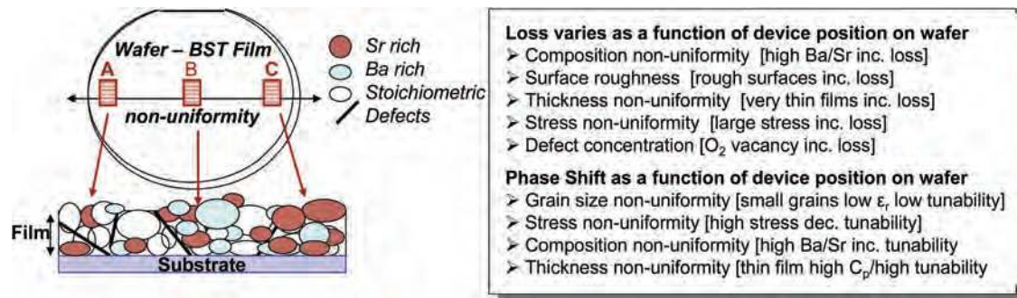
FIG. 33. Schematic diagram showing (a) the film compositional and microstructural non-uniformities and (b) their effects on the phase shifter device properties (Courtesy of M. W. Cole research group, Army Research Laboratory 2012).
