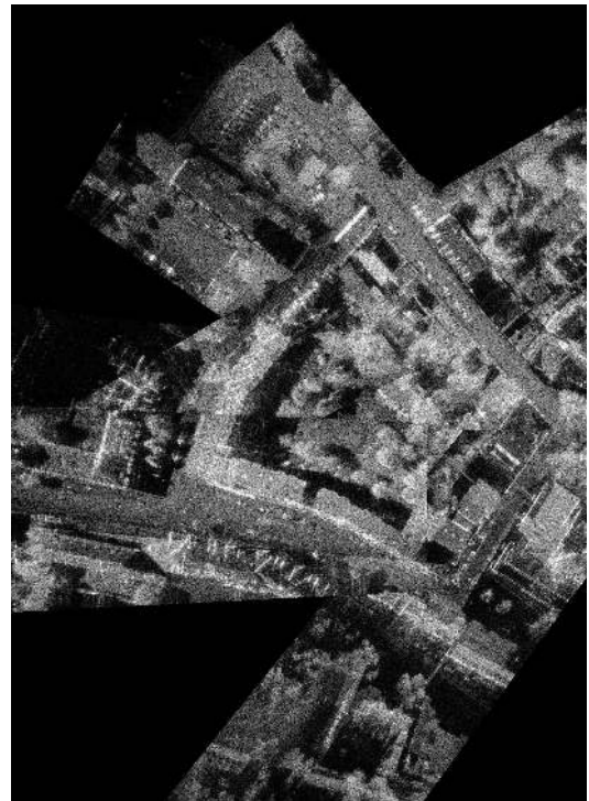
(a) SAR image composed of different aspect angles views
